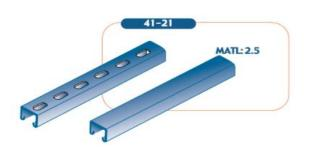
Manufactured in accordance to BS6946 1988 Available with Slots 28x14mm or 28x12mm at 50mm c/c. Lengths - 3m or 6m
