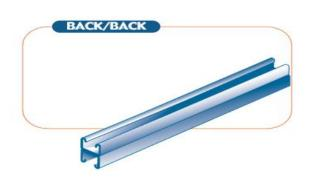
Manufactured in accordance to BS6946 1988 Available with Slots 28x14mm or 28x12mm at 50mm c/c. Lengths - 3m or 6m Spot welded at 150mm c/c
