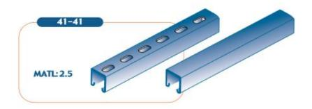
Manufactured in accordance to BS6946 1988 Available with Slots 28x14mm or 28x12mm at 50mm c/c. Lengths - 3m or 6m
